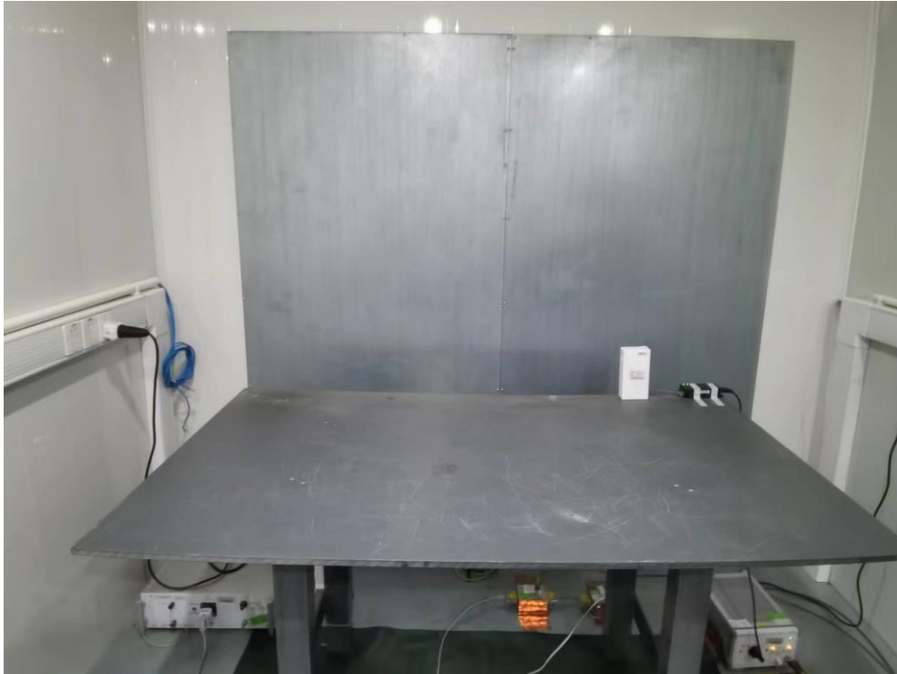
AC Power Line Conducted Emissions Test Photos
