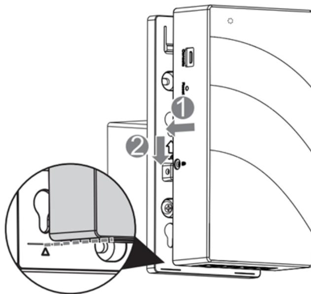
(5) Use a torx screwdriver to lock the torx screw to the anti-theft lock on the side of the AP.
