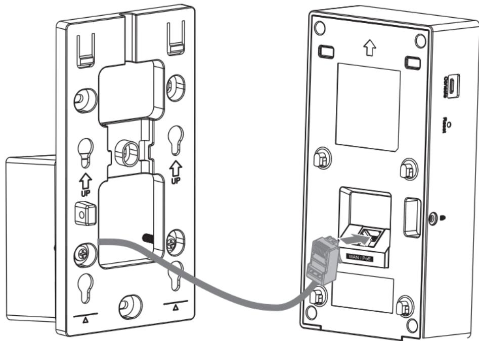
(4) Secure the device with the optical fiber connected to the mounting bracket by using the hooks delivered with the device. During installation, align the hooks with round holes on the mounting bracket and buckle them from up to down.
