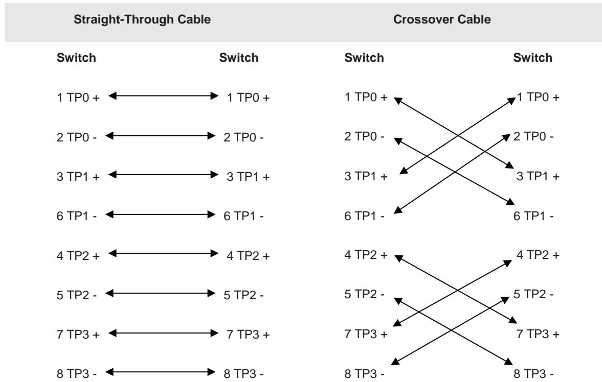
In addition to cables with the above-mentioned specifications, the 100BASE-TX/10BASE-T port can be connected using 100-ohm CAT-3, CAT-4, and CAT-5 cables for at 10 Mbps data speed or using to 100-ohm CAT-5 cables for at 100 Mbps data speed with a maximum connection distance of 100 meters. The following table shows 100BASE-TX/10BASE-T pin assignments.
