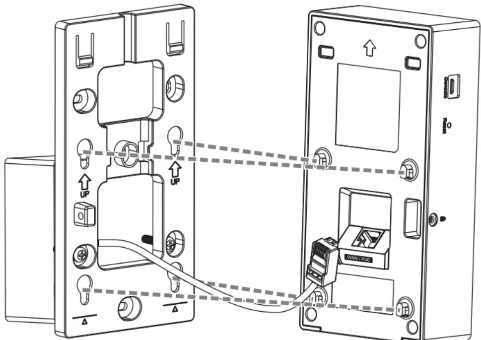
**Figure 3-7** **Installing the AP**
