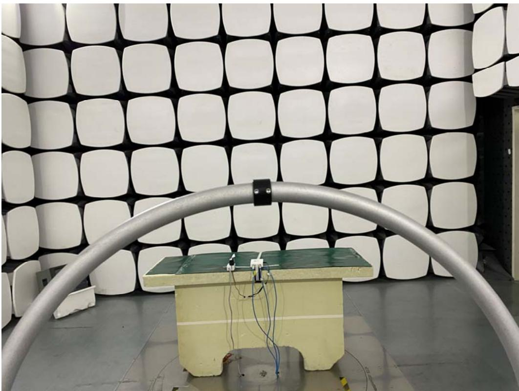
**Radiated Emissions Test Photos****30 MHz to 1 GHz**
