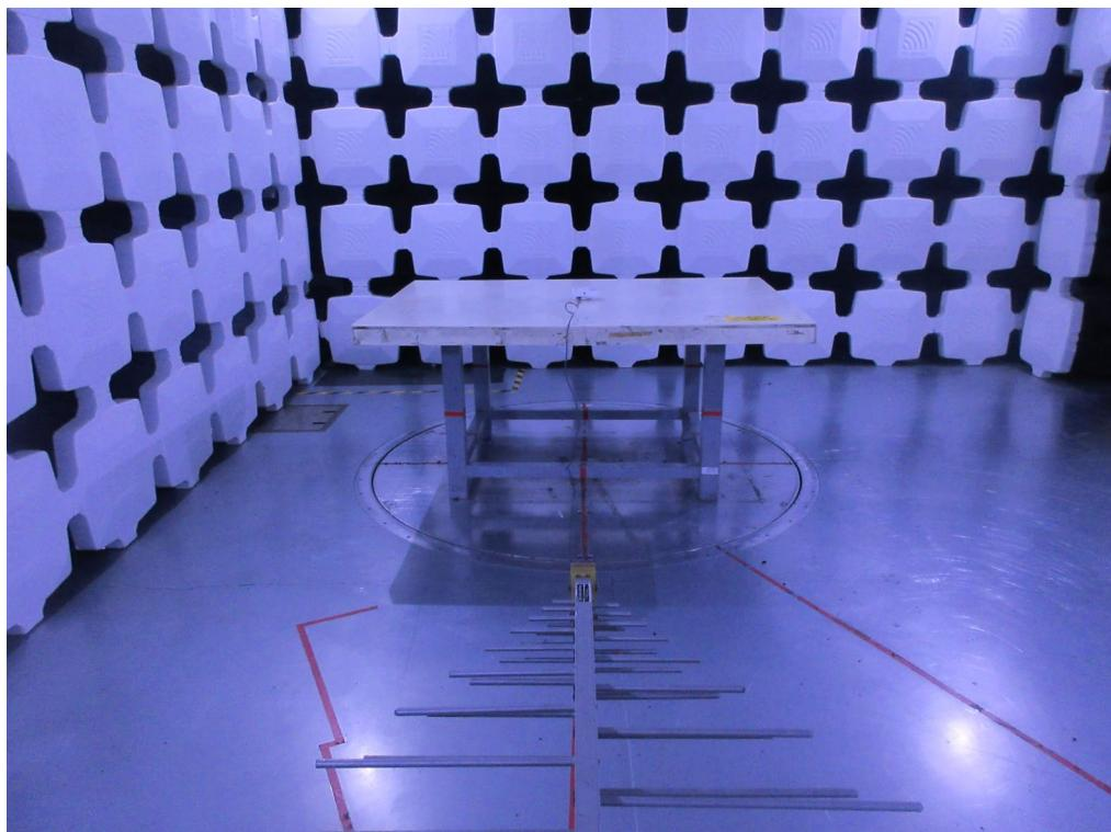
**Radiated Emissions Test Photos****Above 1 GHz**
