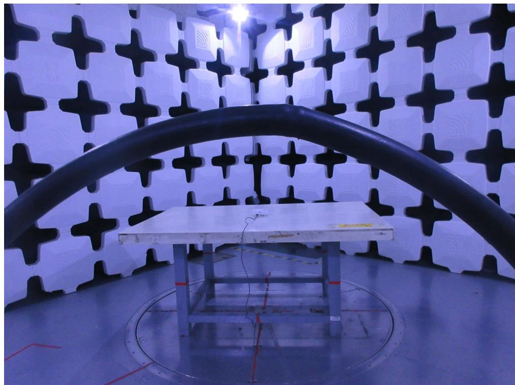
**Radiated Emissions Test Photos****30 MHz to 1 GHz**
