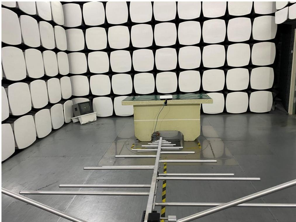
**Radiated Emissions Test Photos****Above 1 GHz**
