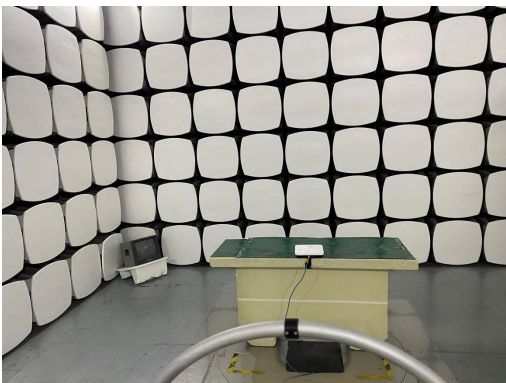
**Radiated Emissions Test Photos****30 MHz to 1000 MHz**
