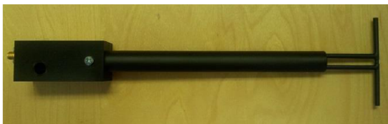
Figure 1 – MVG COMOSAR Validation Dipole
