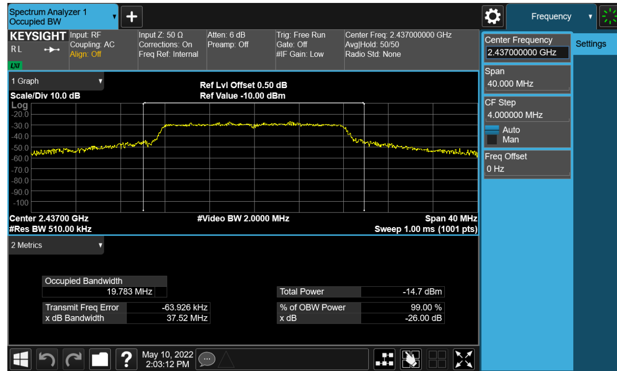
Figure 13: 99% Bandwidth, 802.11g, 2437MHz
