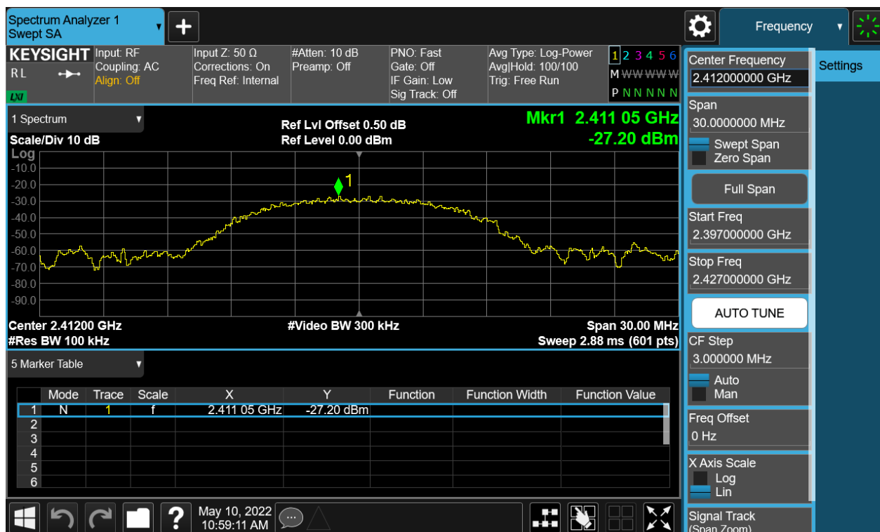
Figure 30: Conducted Spurious Emission & Authorized-band band-edge, 802.11b, 2412MHz Carrier Level
