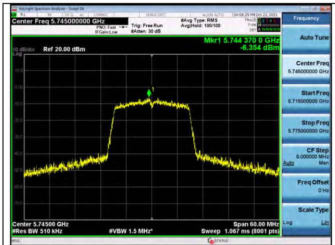
802.11AC20 PSD plot on channel 157
