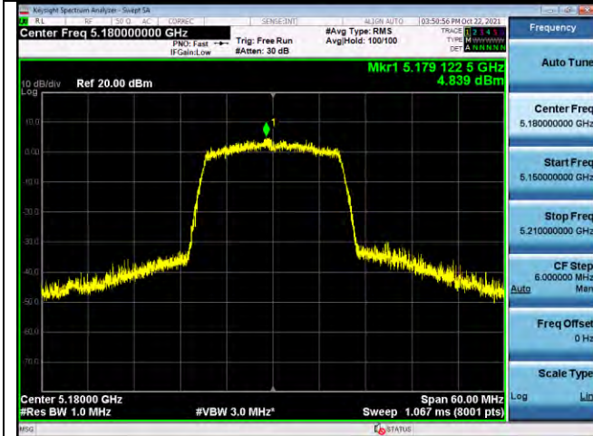
802.11AC20 PSD plot on channel 40
