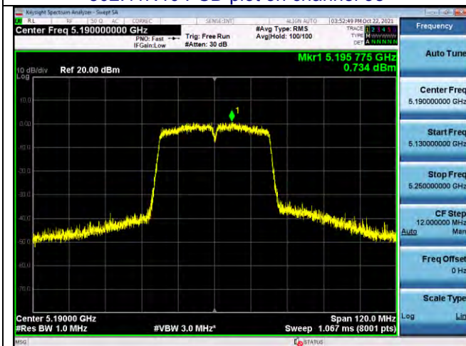
802.11N40 PSD plot on channel 46
