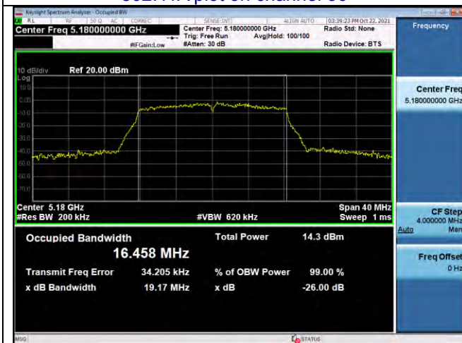
802.11A plot on channel 40
