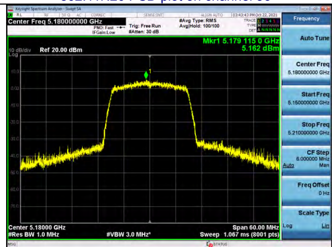
802.11N20 PSD plot on channel 40
