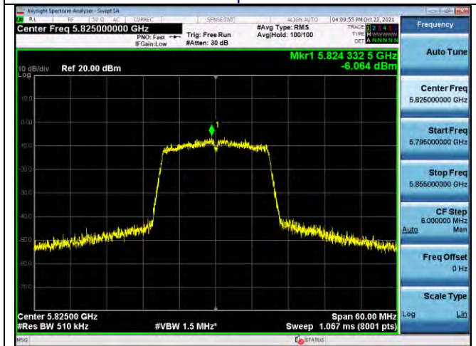
802.11AC20 PSD plot on channel 165
