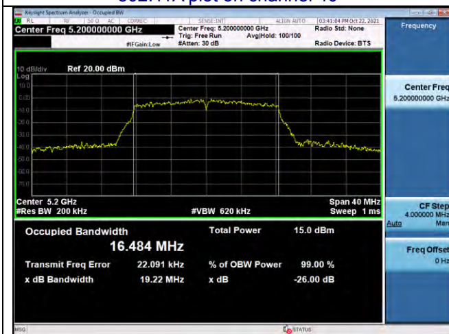
802.11A plot on channel 48
