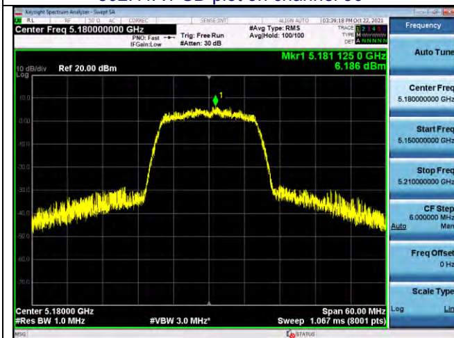
802.11A PSD plot on channel 40
