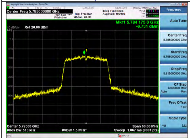
802.11AC20 PSD plot on channel 165
