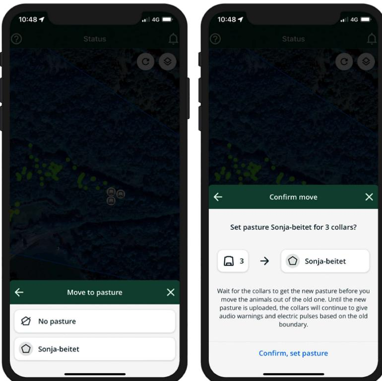
Now, the collars will upload the new pasture they have been assigned to. You can track the process by clicking on the status line on the top of the screen. The info box will appear and let you know if the collars are loading, if they succeed or fail to load, and if the collars have been registered inside their new pasture. The virtual fence will be activated as soon as a collar has registered a position inside the new pasture.
