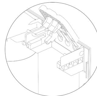
Push the levers up to install filter cartridges.
