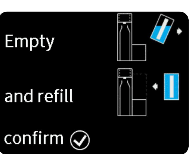
The machine will now ask you to place an empty Clean water container in the beverage tray. Insert the container and press
