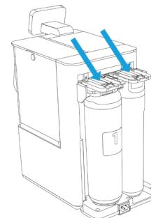
Install the two filter cartridges.
