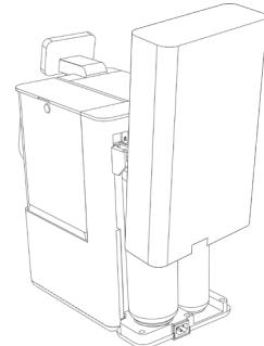
Open the rear cover. Lift up to unlock hooks.
