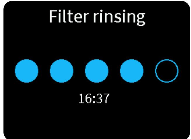
After the rinsing procedure has finished, the machine will ask to empty the clean water container and press
