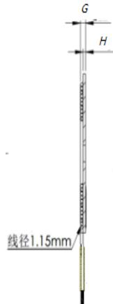
Note: Wrap 8MM (ref) high-temperature adhesive paper around the coil outlet position, and attach double-sided adhesive on the back of magnetic sheet.
