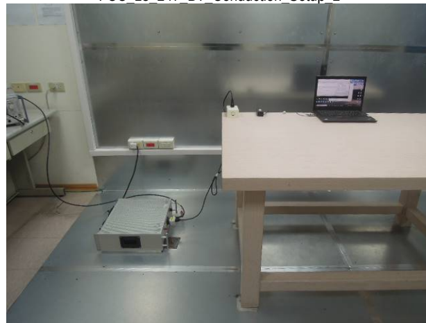
FCC 15 247 BT Conduction Setup 2
