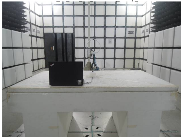
FCC 15 247 BT Radiated Setup 2
