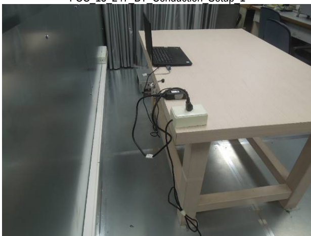
FCC 15 247 BT Conduction Setup 1
