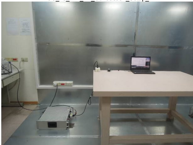
FCC 15 247 BT Conduction Setup 1
