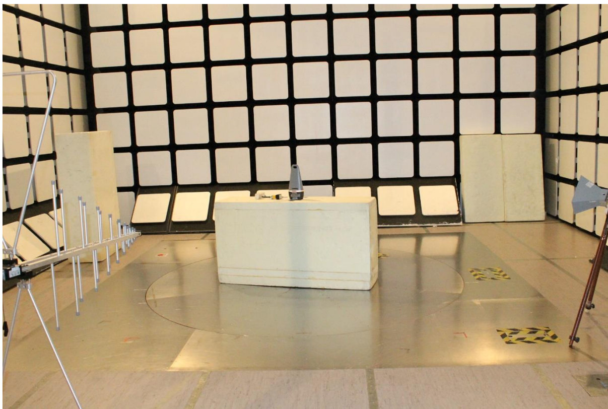
Photograph 1: Radiated spurious emissions setup 30 MHz – 1000 MHz
