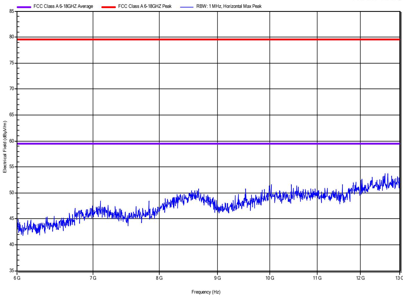
**Radiated RF Emission Measurements – Horizontal Polarisation - Frontside - 13 to 18 GHz**
