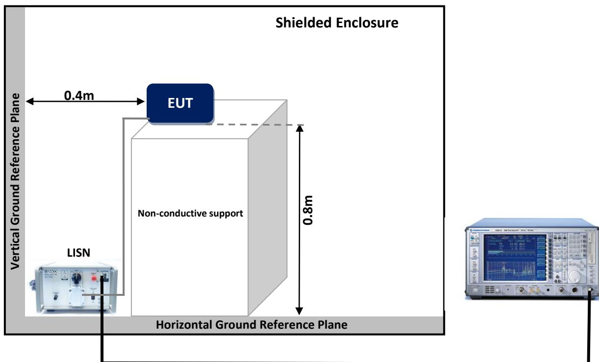
Mains Terminal Emissions measurement setup photos.
