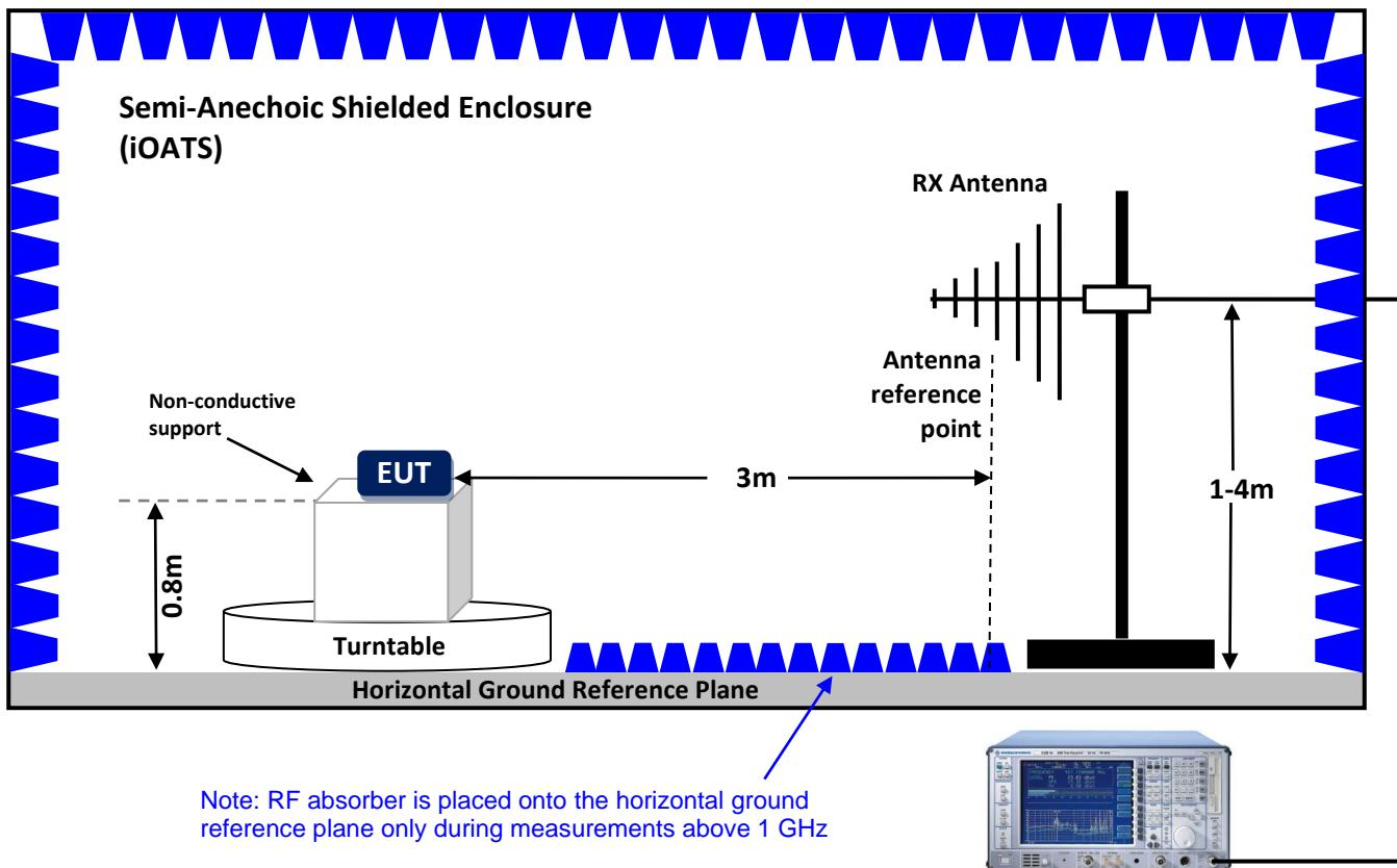
Radiated RF emissions measurement setup photos.
