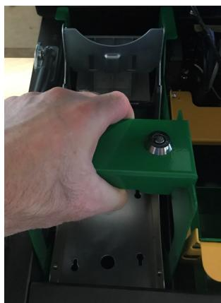
STEP 8 Hold the BNA Lock Bracket as shown.
