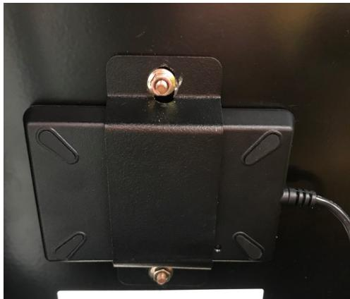
STEP 4 Remove & retain 2x Nuts and 1x Bracket fastening the NFC Reader from the underside of the Top Lid.
