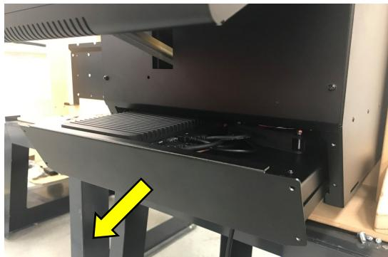
STEP 4 The PC Tray travel is limited by the Main Loom length.
