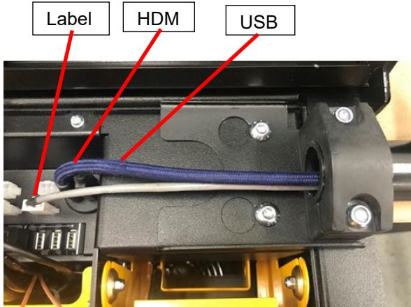
STEP 2 Unplug 3x LCD Screen Loom plugs from the USB Hub.
