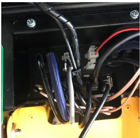
STEP 3 Remove the NFC Reader USB connector from the applicable USB Port.
