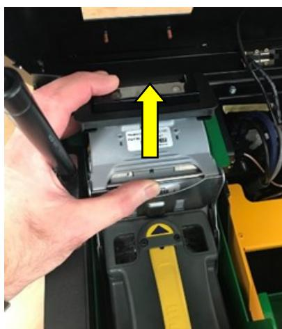
STEP 3 Hold the Bill Validation Module and gently lift the steel rod upwards to disengage & remove from the BNA Bracket.
