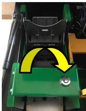
STEP 7 Re-close the BNA Lock Bracket and lock.
