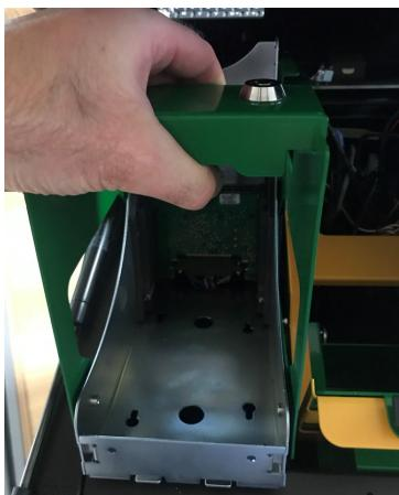
STEP 9 Lift & tilt the BNA Mount Bracket upwards to clear the underside of the Top Lid & Kiosk Main Frame.
