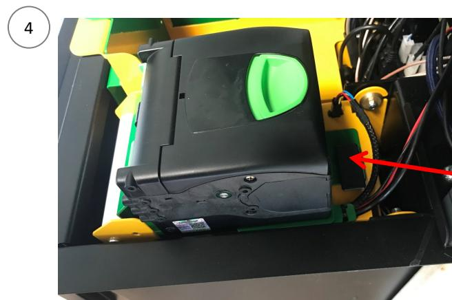
STEP 4 Undo the Latch Swell to disengage the green printer tray.
