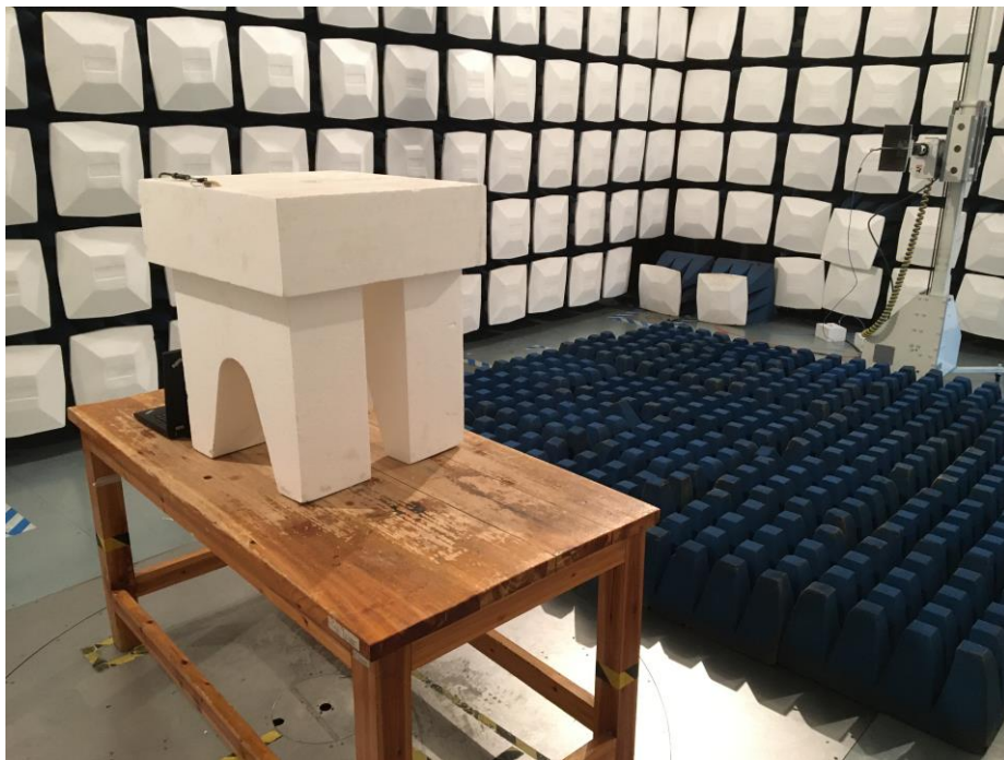
Test Setup For Radiated Emission (Above 1GHz)
