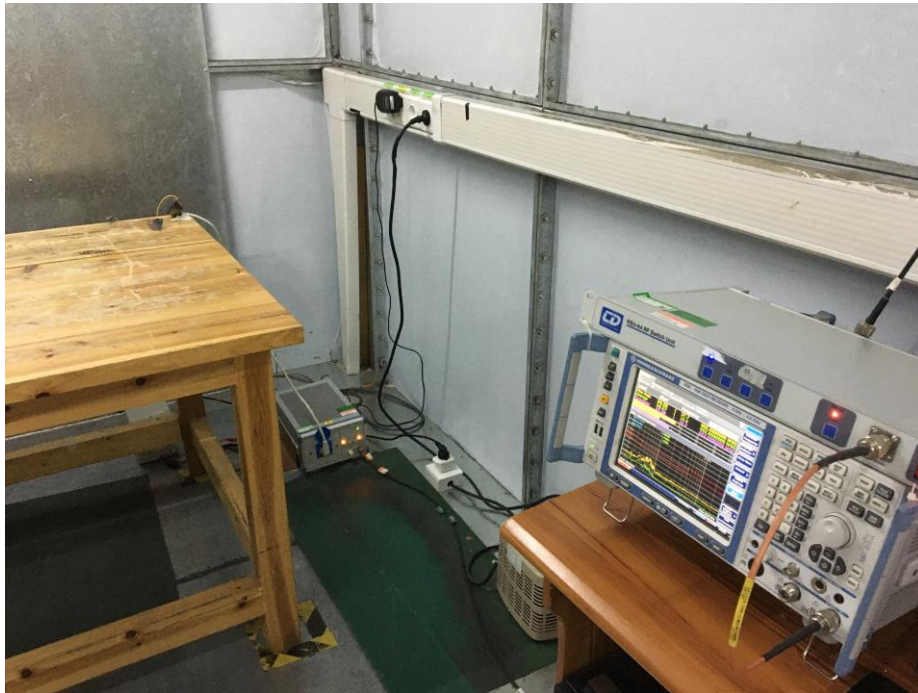
Test Setup For Conducted Emission
