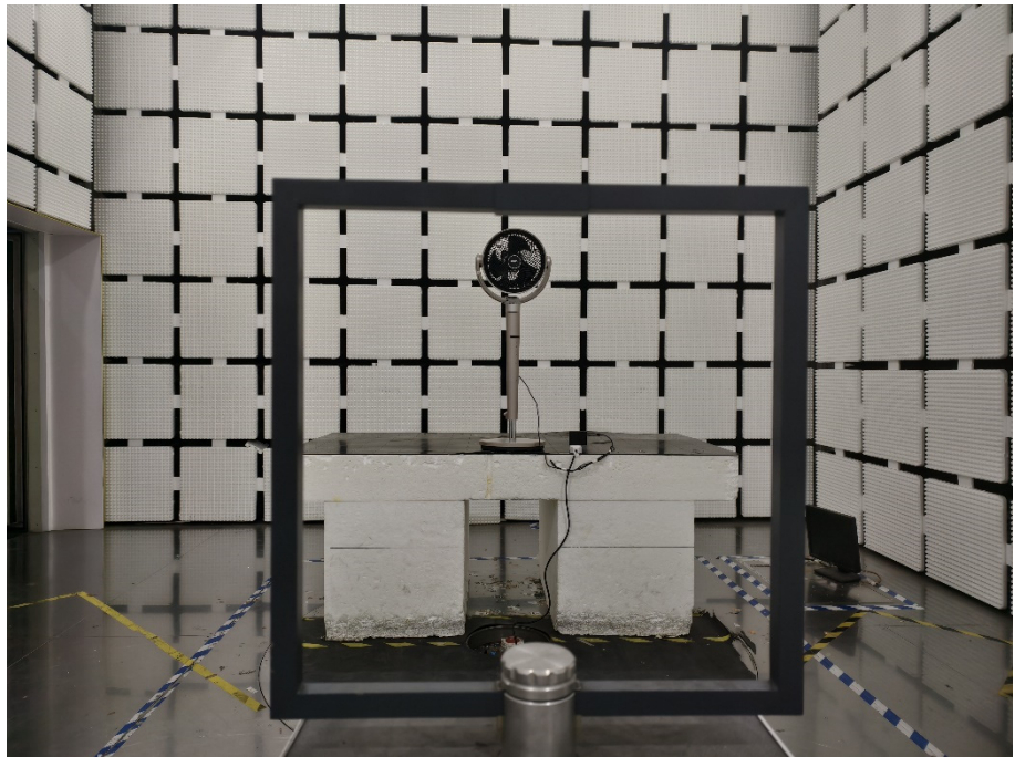
Radiation Emission Test Setup (Below 30MHz)
