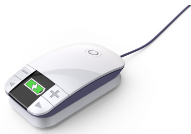
Figure 4. NiNA is fully charged when the battery icon is completely green
