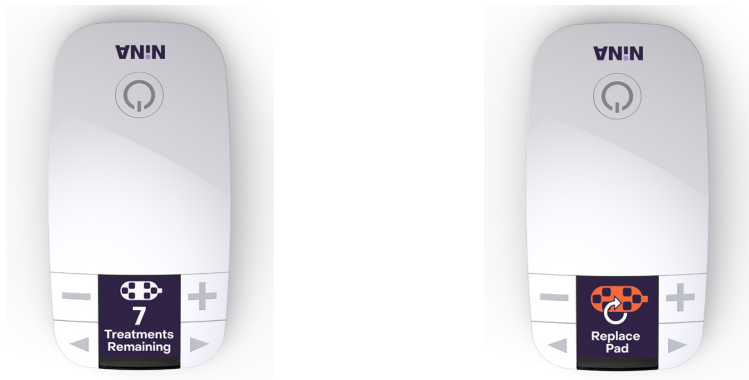
Figure 15. The NiNA display will show the Pad status. Replace the Pad if the Replace Pad alert is displayed.
