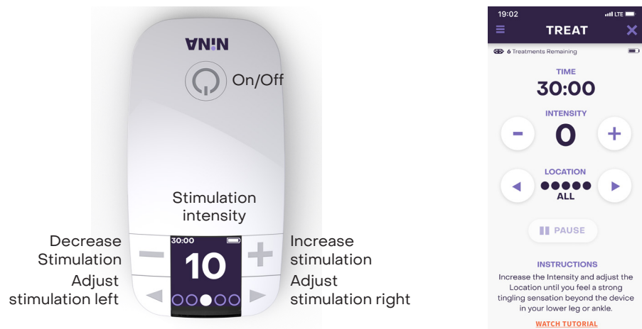
Figure 18. The stimulation intensity and location can be controlled with the +, -, <, and > buttons on NiNA or the NiNA App. Adjust the buttons to find the setting that produces the strongest, yet comfortable stimulation down the leg into the ankle or foot.
