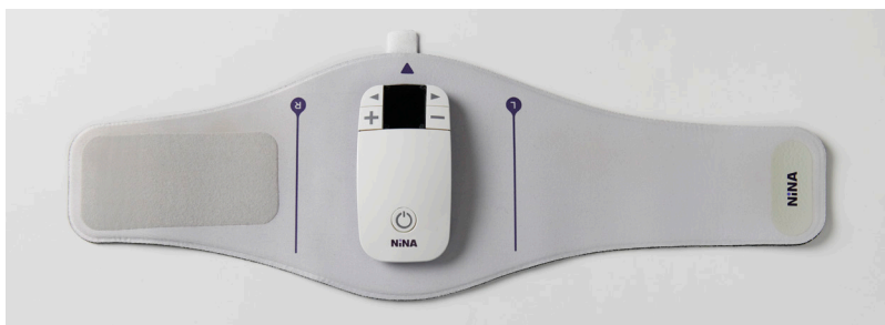
Figure 8. The assembled NiNA, Pad, and Wrap
