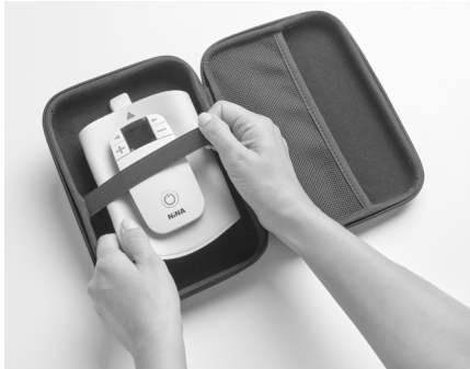
Figure 24. Fold the arms of the Wrap around the Pad and optionally store in the NiNA Case
