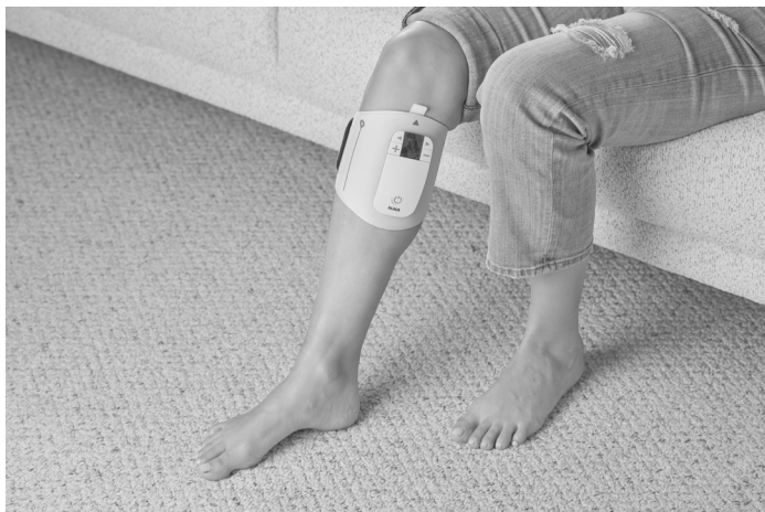
Figure 2. NiNA is placed on the inside of the leg just below the knee crease.
