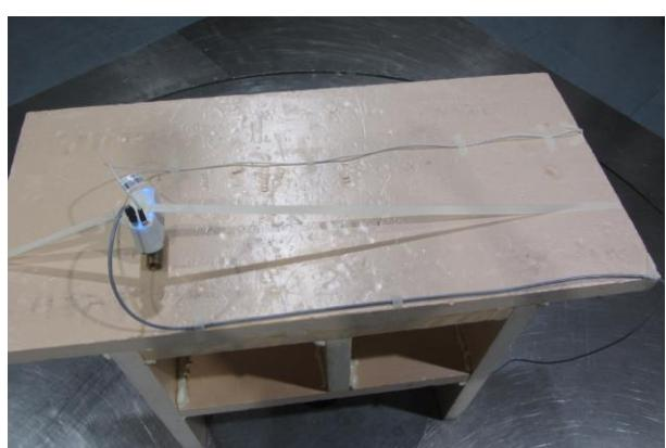
**Setup photo for testing according KDB996369**
