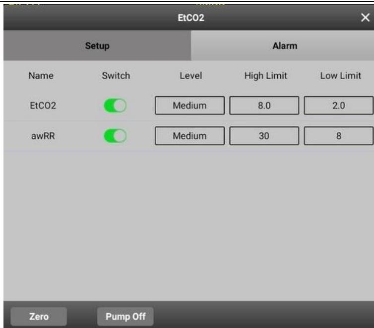
Figure 9-3 EtCO2 Alarm Setup Menu
