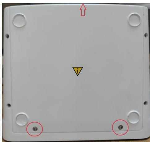
Figure 3-1 Battery compartment cover
