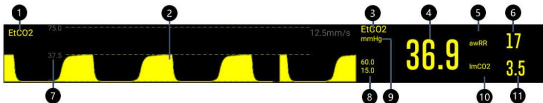
Figure 13-1: EtCO<sub>2</sub> Waveform and Parameter Display
