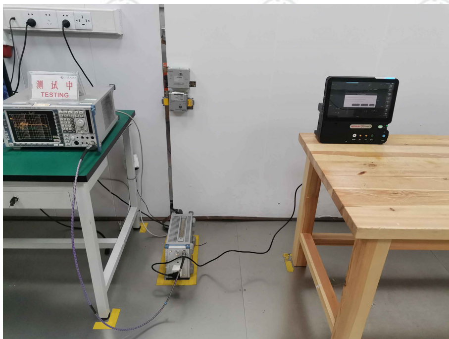
Conducted Emissions Test Setup
