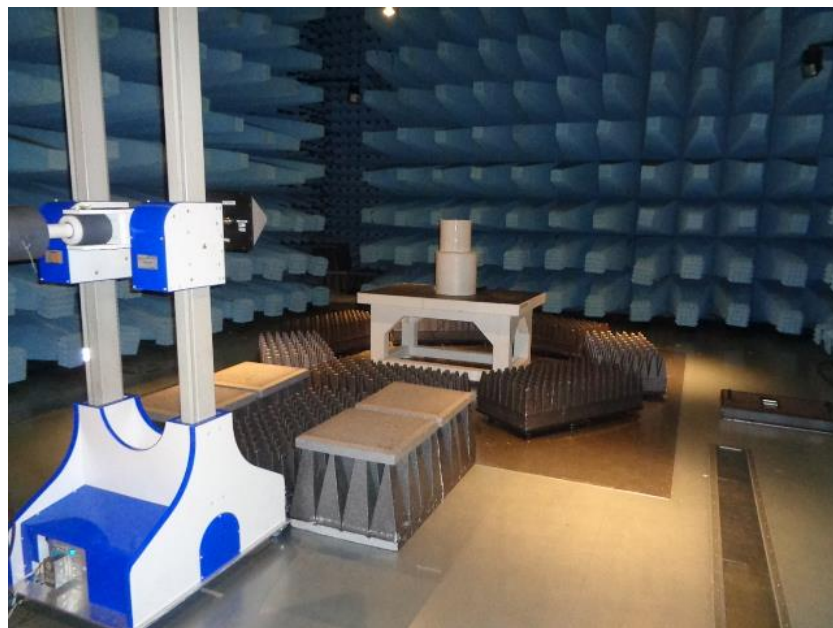
Figure 9.1-2: Radiated emissions set-up for frequencies above 1 GHz
