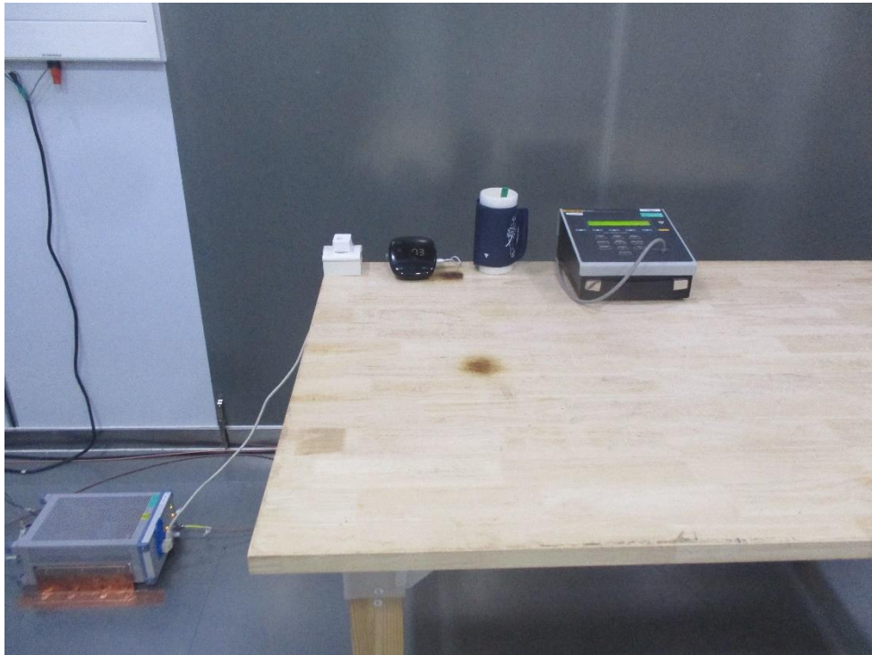
Radiated Emission test of 30MHz-1GHz
