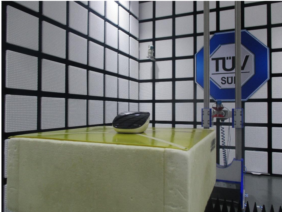
Radiated Emission test 18-25GHz
