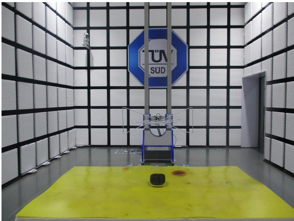
Radiated Emission test of 30MHz-1GHz
