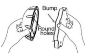
② Put the three bumps on the tooling into the three round holes of iBeacon battery cover
