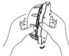
③ Turn the tooling counterclockwise to open the battery cover
