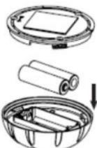
⑤ Put in two new No. 5 batteries and replace the battery cover
