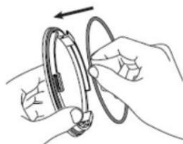
④ (optional) take out the battery cover and put the sealing ring on the battery cover
