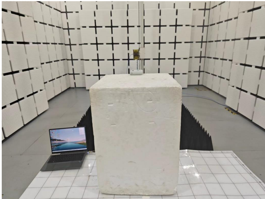
Set-up for Radiated Spurious Emission, Above 1GHz
