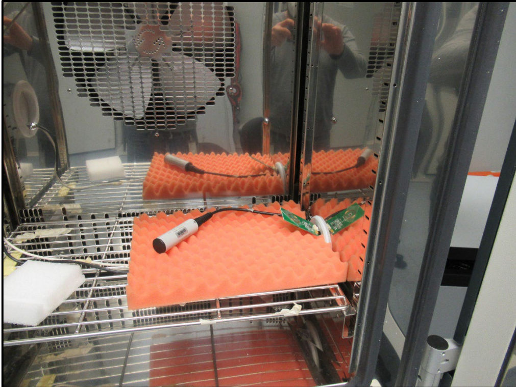
Photo 5: Frequency Stability & Bandwidth Test Setup
