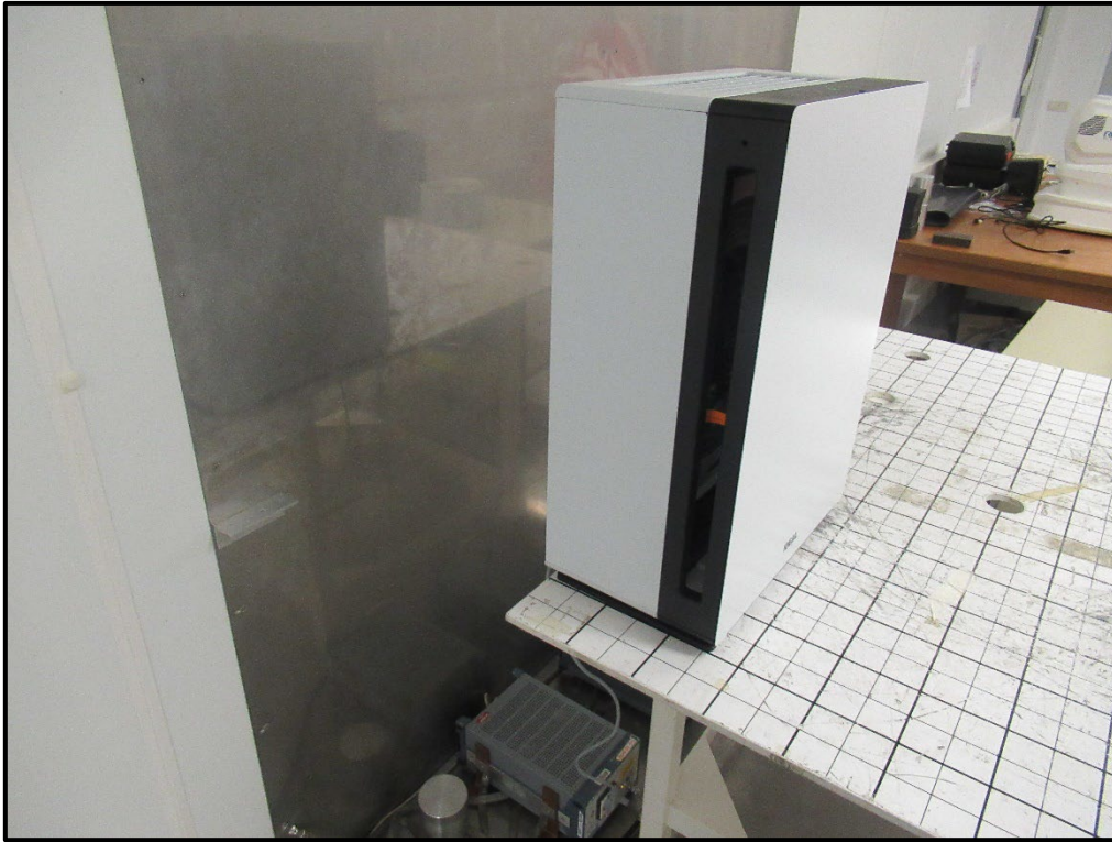
Photo 7: AC Conducted Emissions Test Setup
