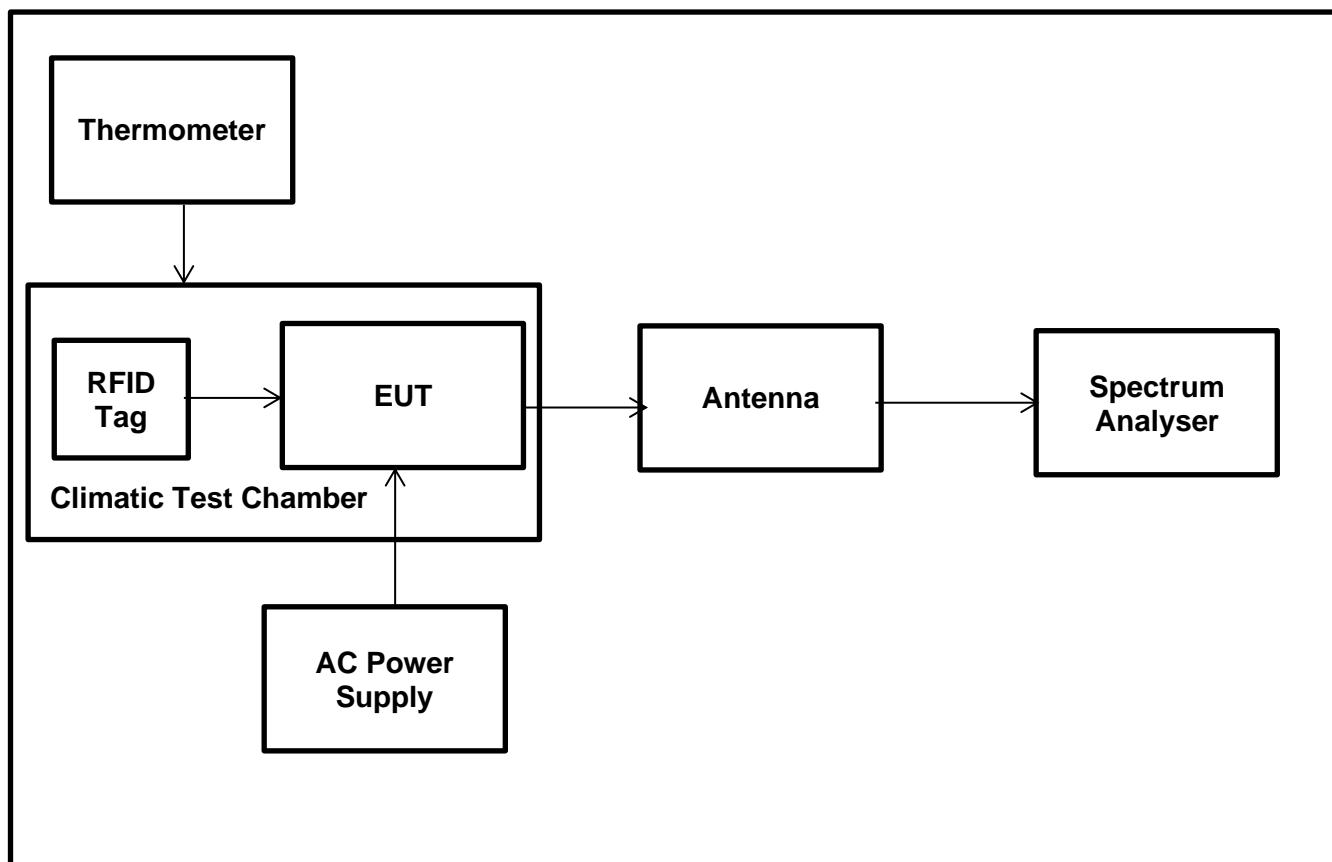
**Transmitter Frequency Stability (Temperature & Voltage Variation) (continued)****Results: AC Power supply / RFID 13.56 MHz / Temperature Variations**
