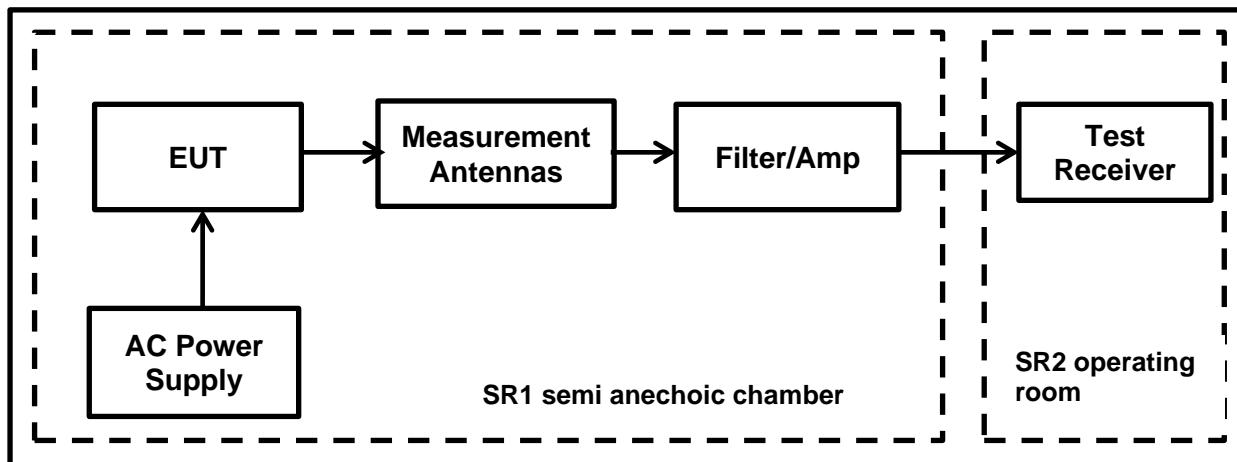
**Transmitter Radiated Emissions (continued)****Results: AC Power supply / RFID 13.56 MHz**
