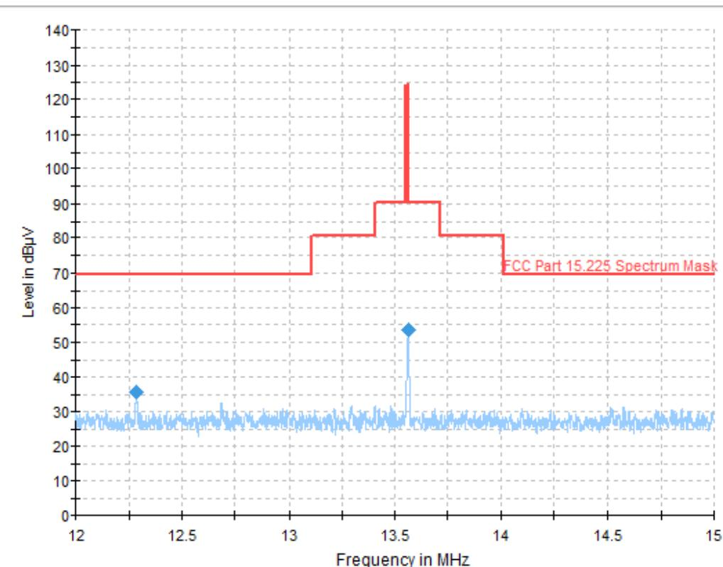
Fundamental field strength and spectrum mask / measured at 3 metres in a semi-anechoic chamber
