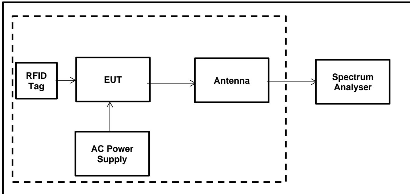
**Transmitter 20 dB Bandwidth (continued)****Results: AC Power Supply / RFID 13.56 MHz**
