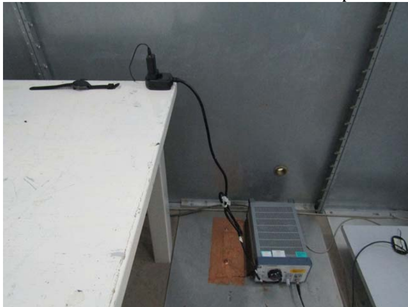
Measurement of Conducted Emission Test Set Up
