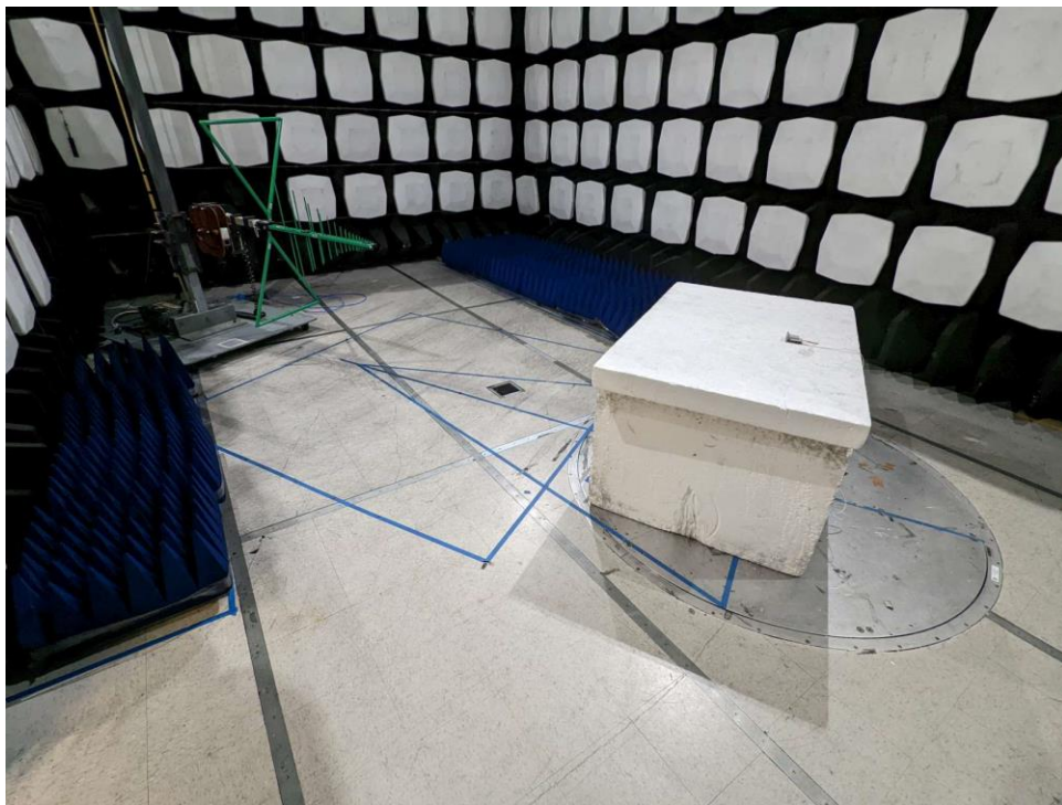
Figure A-2: Test Setup – Radiated Emissions <1GHz
