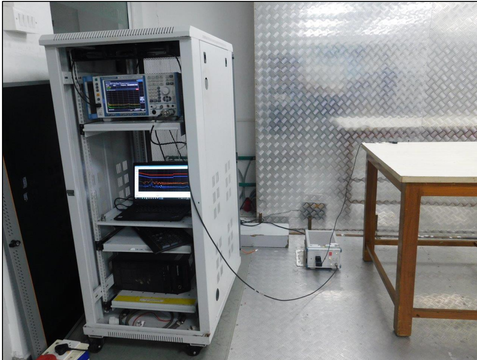
Conducted emission test setup
