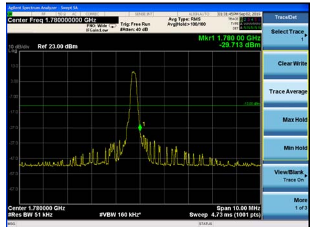
LTE Band 66 16QAM 1.4MHz CH-High, 100%
