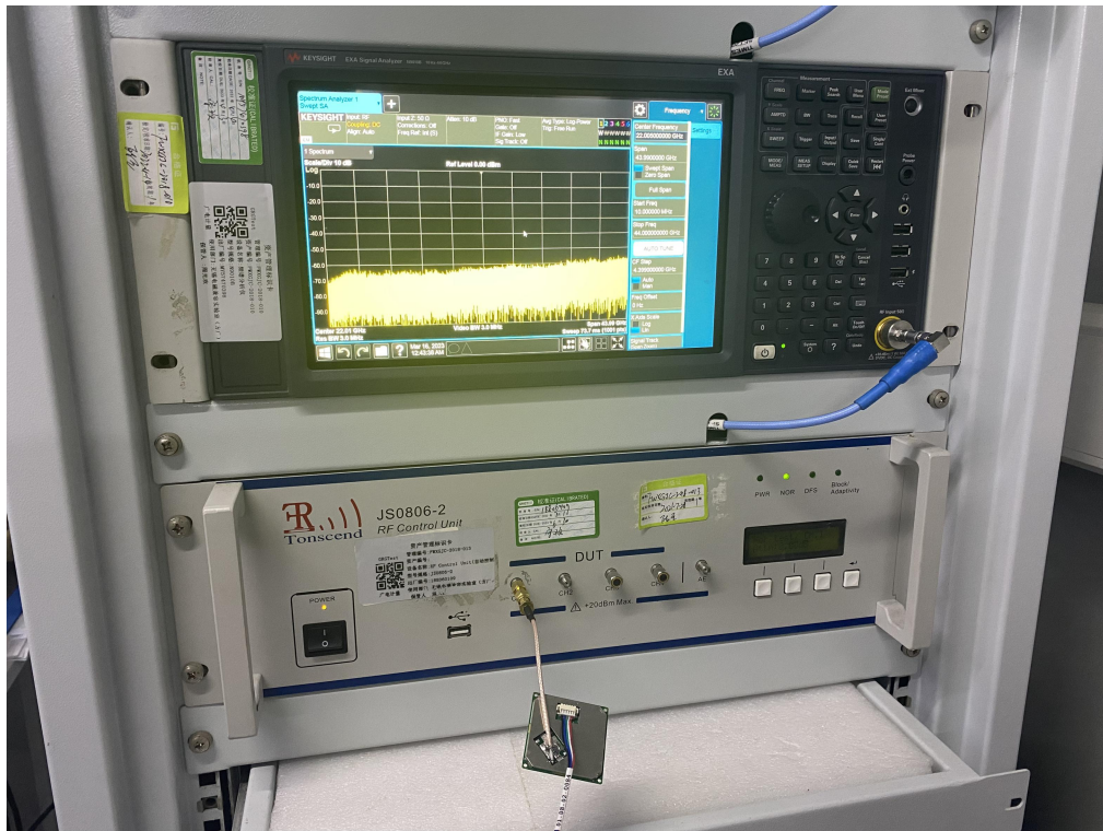
Description: Conducted Test Setup Photo
