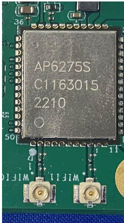
Photo 5: Internal View for WiFi&BT Module
