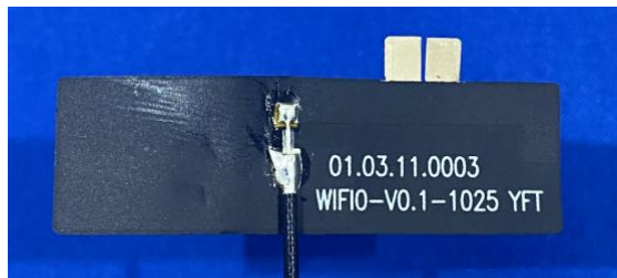
Photo 9: Internal View for BT&WIFI0 ANT
