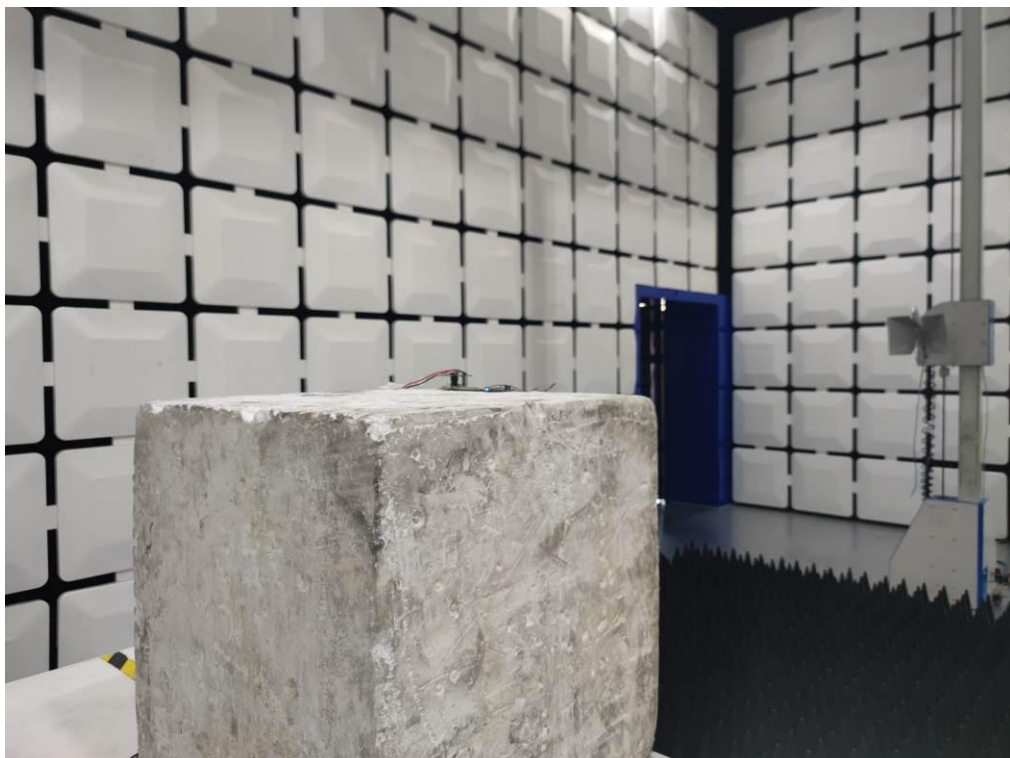
Description: Radiated Emission Test Setup for Above 1GHz
