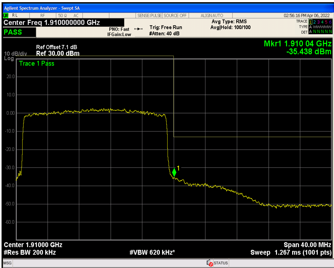
Band2 QAM16 BW=20MHz Channel=19100 RB Size=100 Position=#0
