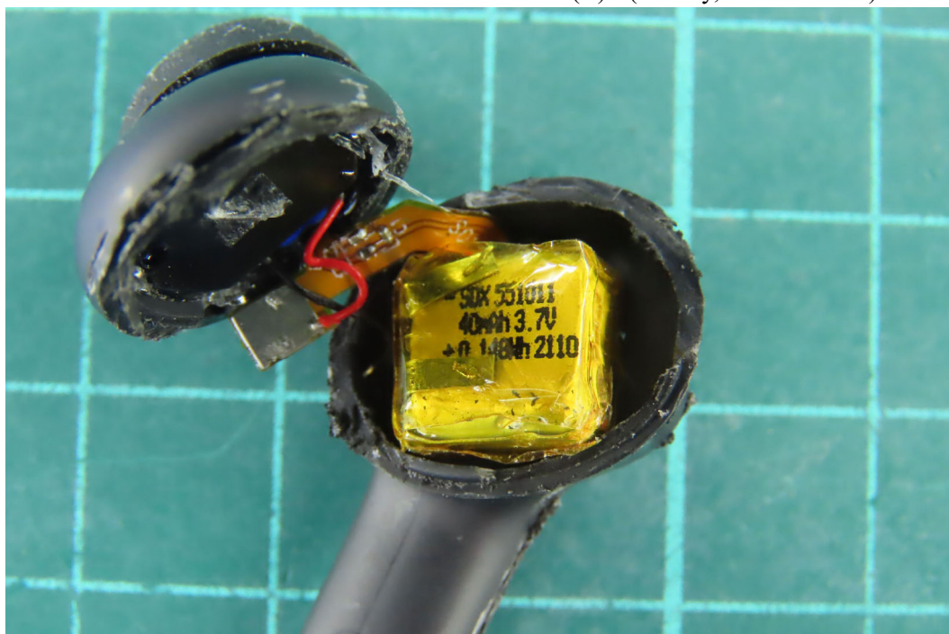
(8) EUT Photo - M/N: ROG CETRA TRUE WIRELESS(R) - (Battery, M/N: 551011)
