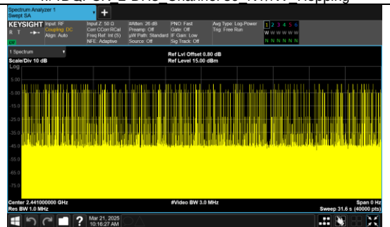
Number of Pulses in 31.6 seconds π/4DQPSK 2-DH5 Channel 39 NT/NV Hopping
