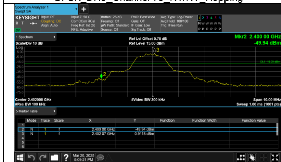
Out Of Band Emission pi/4DQPSK 2-DH5 Channel 0 NT/NV
