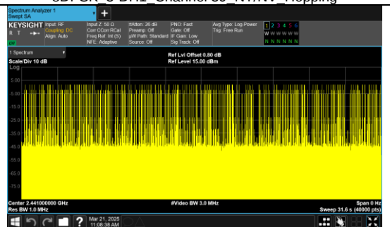
Number of Pulses in 31.6 seconds 8DPSK 3-DH3 Channel 39 NT/NV Hopping
