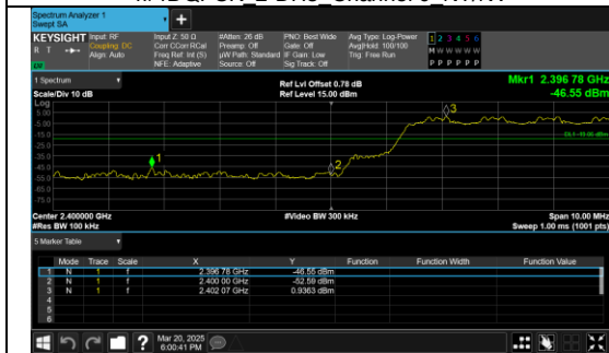
Out Of Band Emission(Left) pi/4DQPSK 2-DH5 Channel 0 NT/NV Hopping
