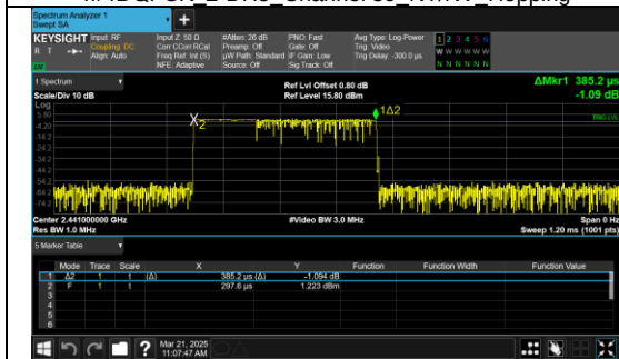
Pulse Width 8DPSK 3-DH1 Channel 39 NT/NV Hopping
