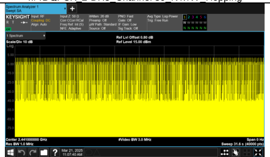
Number of Pulses in 31.6 seconds 8DPSK 3-DH1 Channel 39 NT/NV Hopping
