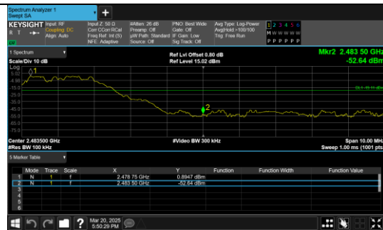
Out Of Band Emission(Right) GFSK DH5 Channel 78 NT/NV Hopping
