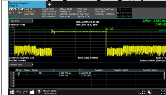
Pulse Width GFSK_DH5_Channel 39_NT/NV_Hopping
