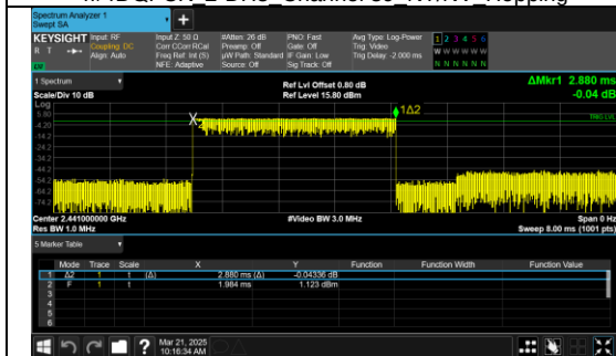
Pulse Width π/4DQPSK 2-DH5 Channel 39 NT/NV Hopping
