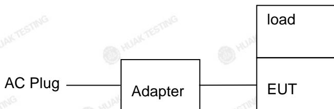
Operation of EUT during radiation testing:
