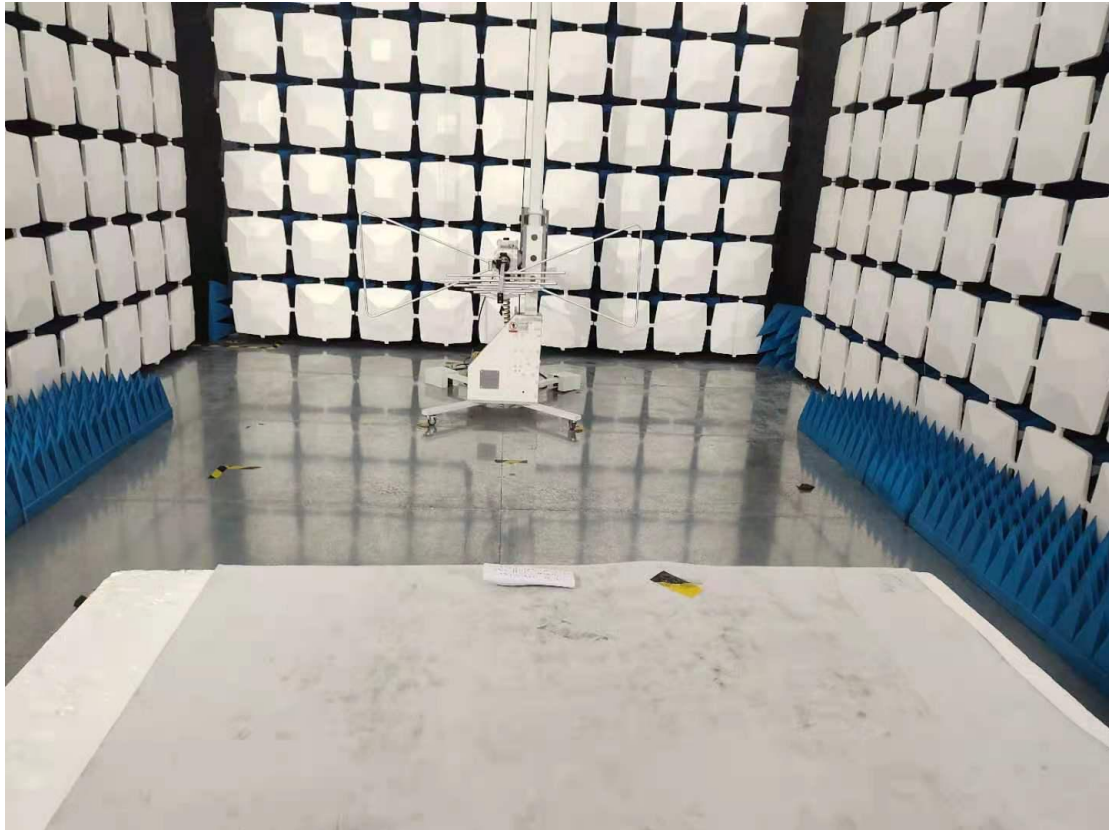
Above 1GHz for radiated emission test setup
