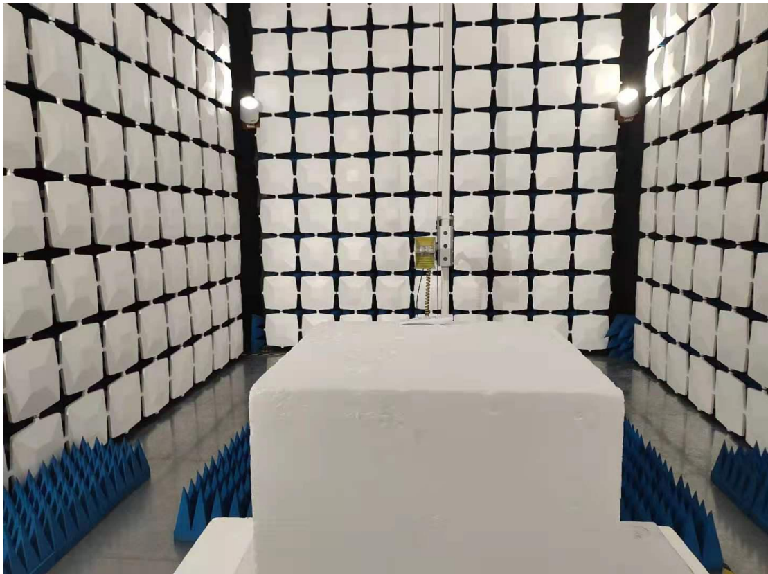
Above 1GHz for radiated emission test setup
