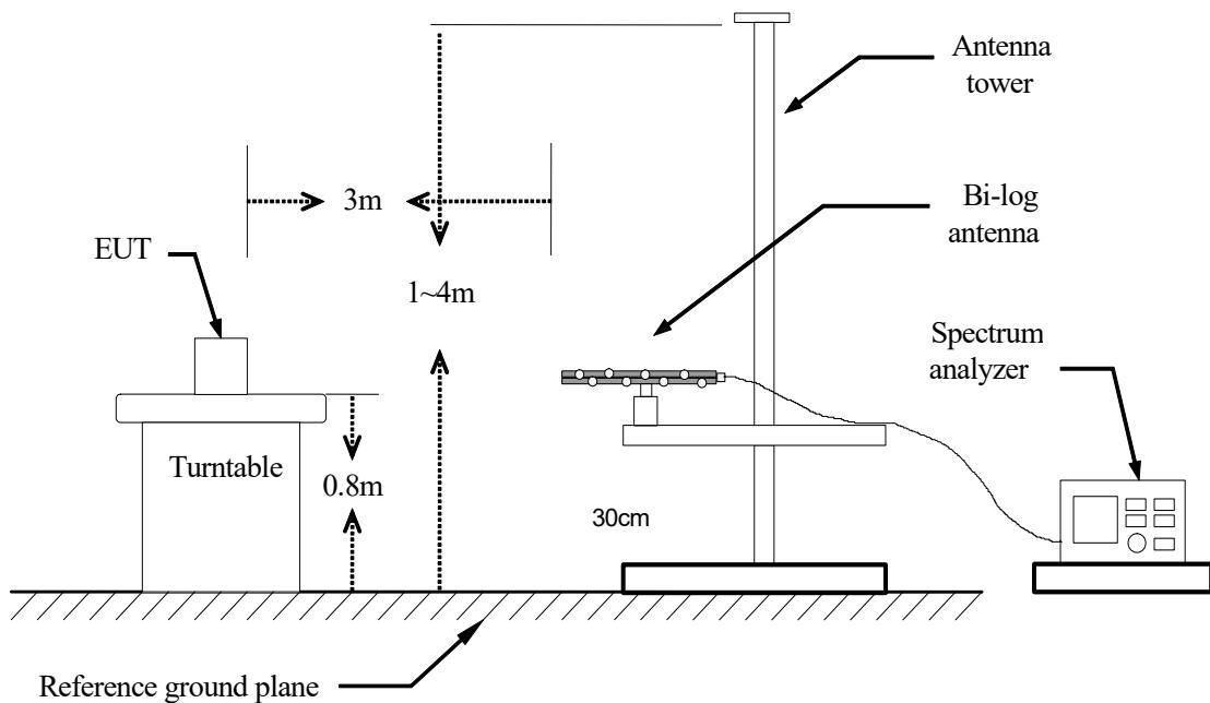
**Above 1 GHz**
