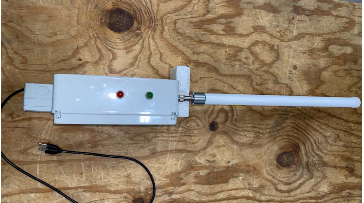
HIFIS Side View with Annunciator LEDs
