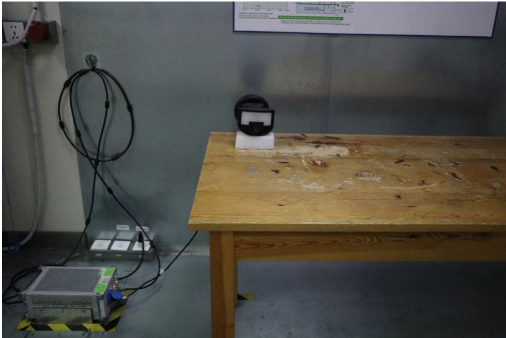
Photograph 3: Set-up for Conducted Emission on AC Mains
