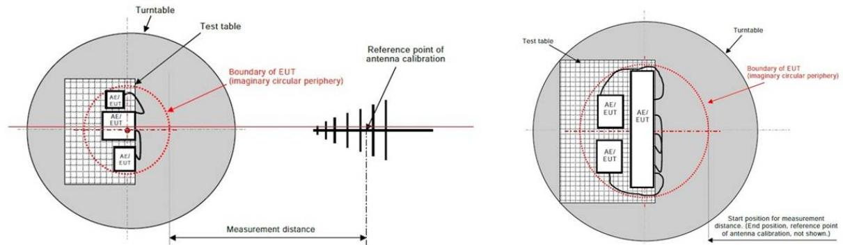
The radiated emission tests were performed in the 3 meters chamber test site, using the setup accordance with the ANSI C63.4-2014. The related limit was specified in FCC Part 15B.
