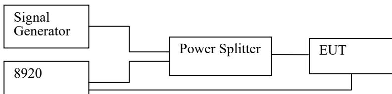
2. Apply a signal to the EUT antenna port at lowest, middle, highest channel frequencies of the operating band;
