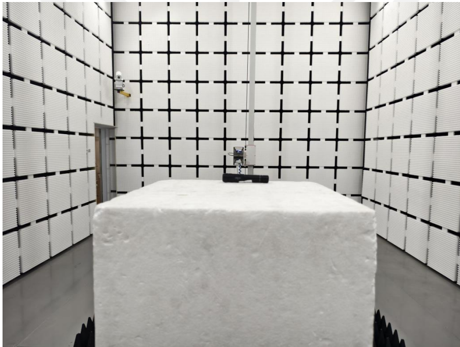
Spurious Radiation Emissions Test (> 1G)
