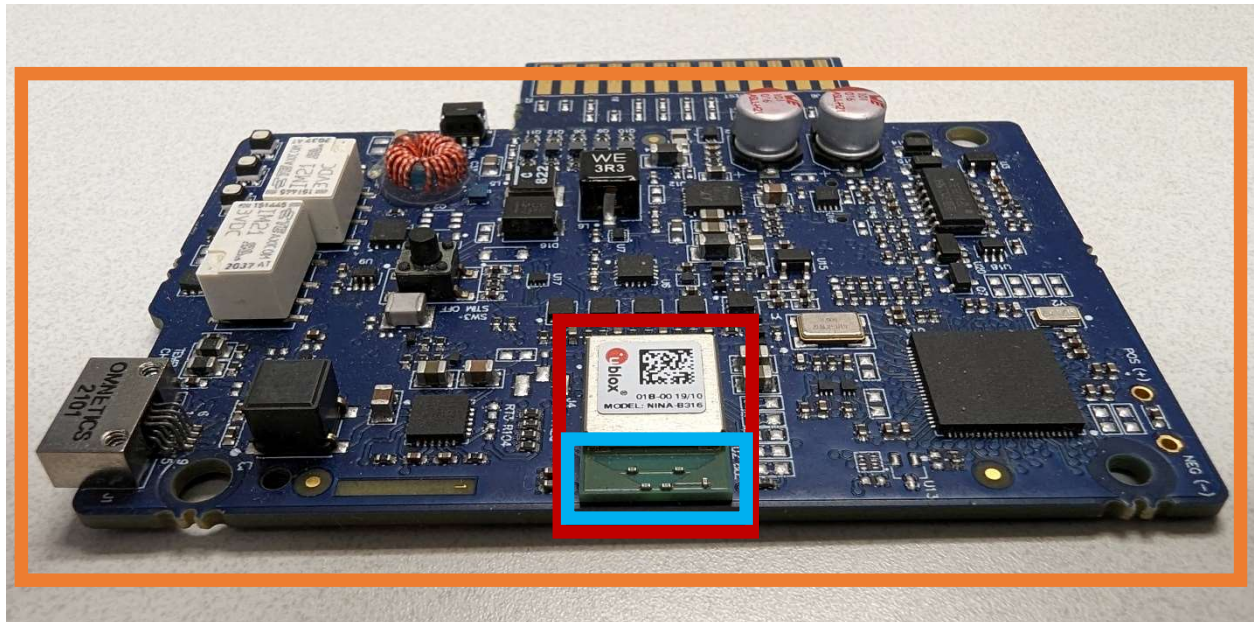
NINA-B3x6 with internal antenna on Charger host board – detail view
