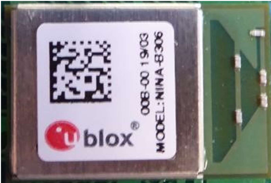
NINA-B3_internal_photo*1: EUT NINA-B3 – with shielding
