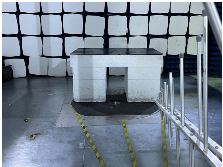
Radiation Emission Test Setup (30MHz to 1GHz)
