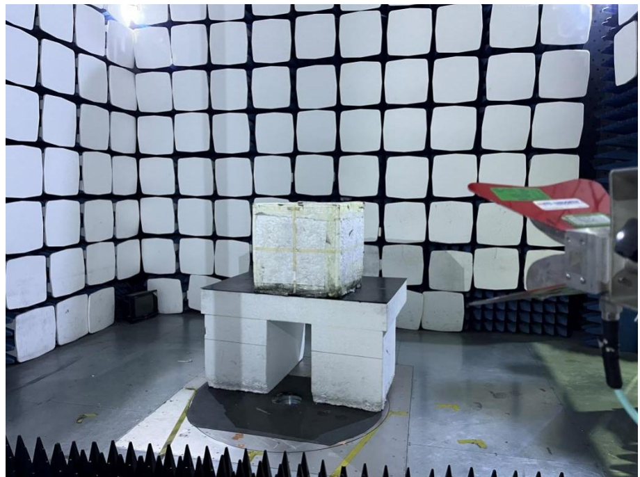
Radiation Emission Test Setup (1GHz to 18GHz)
