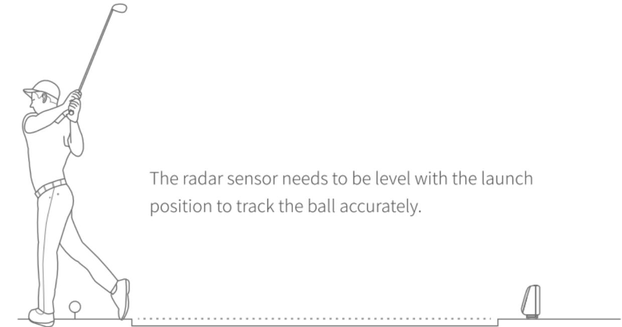
The radar sensor needs to be level with the launch position to track the ball accurately.
