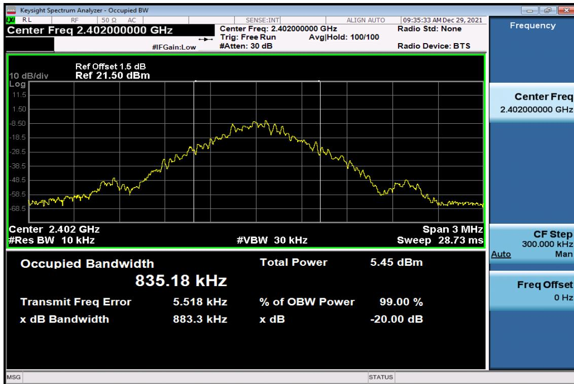
**20dB Bandwidth Test Data CH-Mid**
