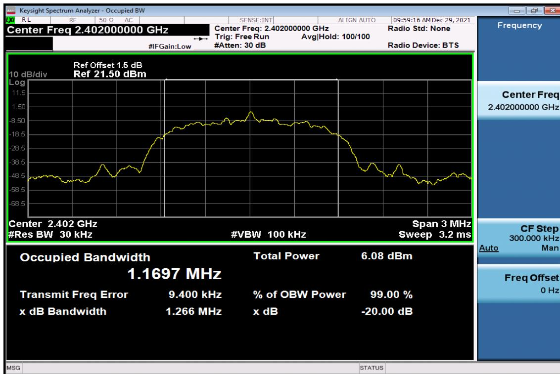
**20dB Bandwidth Test Data CH-Mid**
